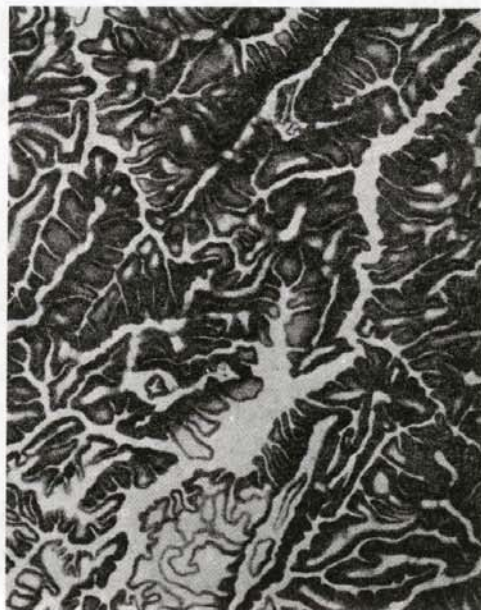
Slope shading. Scale about 1:500,000. Area near Gheorghieni in the Carpathians.
