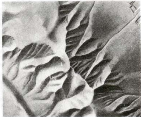
6. Graphically produced relief shading, light from west-north-west.
